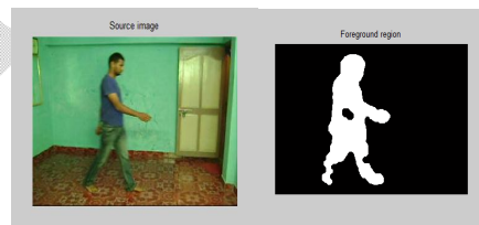
Fig 2 : Result of background subtraction for indoor environment
